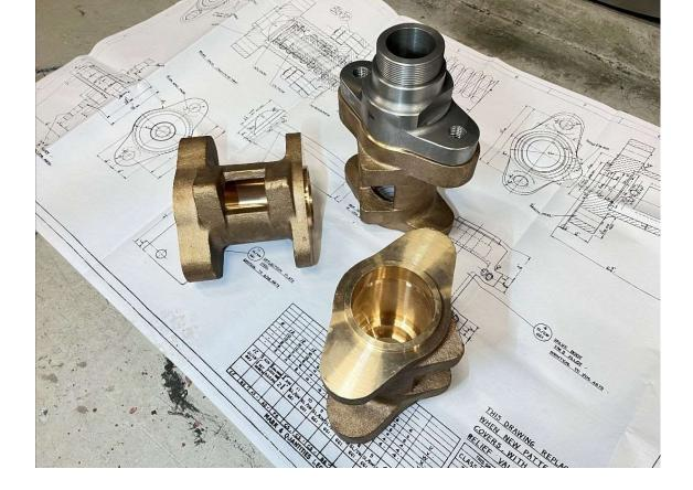
Here and at the top of the page are photos of the cylinder release valves that our apprentice Ed is machining for the P2 at the moment. They fit on the front and back of each cylinder and act as safety valves to release water if the engine carries water over from the boiler.
